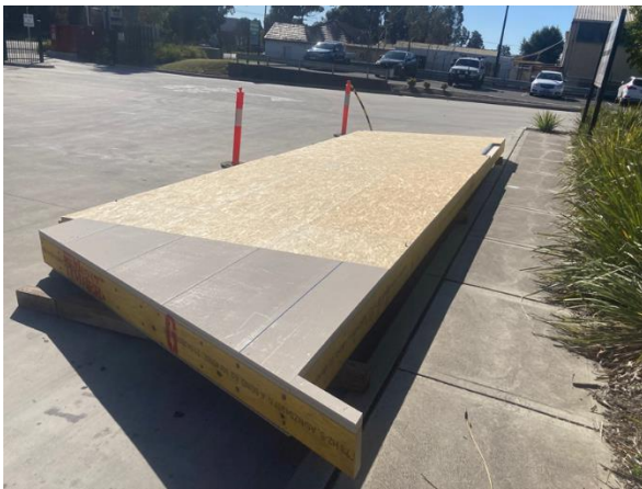
Floor Cassette manufacture Meyer Timber NSW
