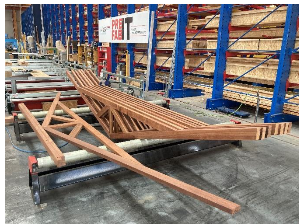
Merbau Trusses fabricated at Meyer Timber
